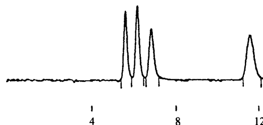
Fig. 3. Chromatogram illustrating the separation of a mixture of racemic ( \pm )-threo and racemic ( \pm )-erythro mefloquine. Column: Chiralpak AD (250 \times 4.6 mm). Mobile phase: hexane-ethanol-diethylamine (96:4:0.1). Flow rate: 1.0 ml/min. Retention times: (+)-( 11R/2'R )-threo, 5.72 min; (-)-( 11S/2'S )-threo, 6.29 min; (-)-( 11S/2'R )-erythro, 6.95 min; (+)-( 11R/2'S )-erythro, 11.67 min.
